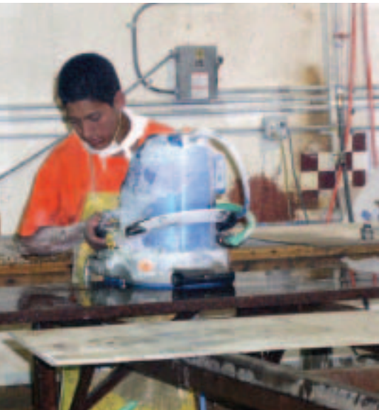
Some of the more complex edging operations are completed with a Marmoelettromeccanica Master 3500 portable edging machine.
