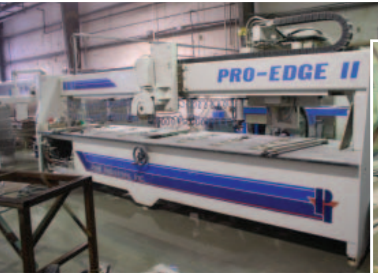
A Pro Edge II from Park Industries is used for automated edge processing.
