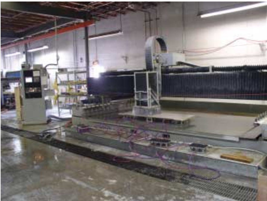
When choosing a CNC machine, the owners of Counter Revolution selected one from Northwood Machine Manufacturing Co. "There are many advantages to buying American technology when it comes to maintenance," said co-owner Leonardo Ventimiglia, adding that the piece of machinery contains a 32-tool changer.
