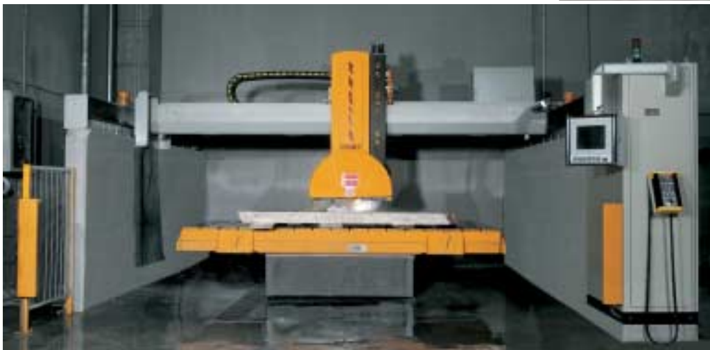
The most recent addition to Counter Revolution's line of equipment is a Breton FRPC 700 numerically controlled saw.
