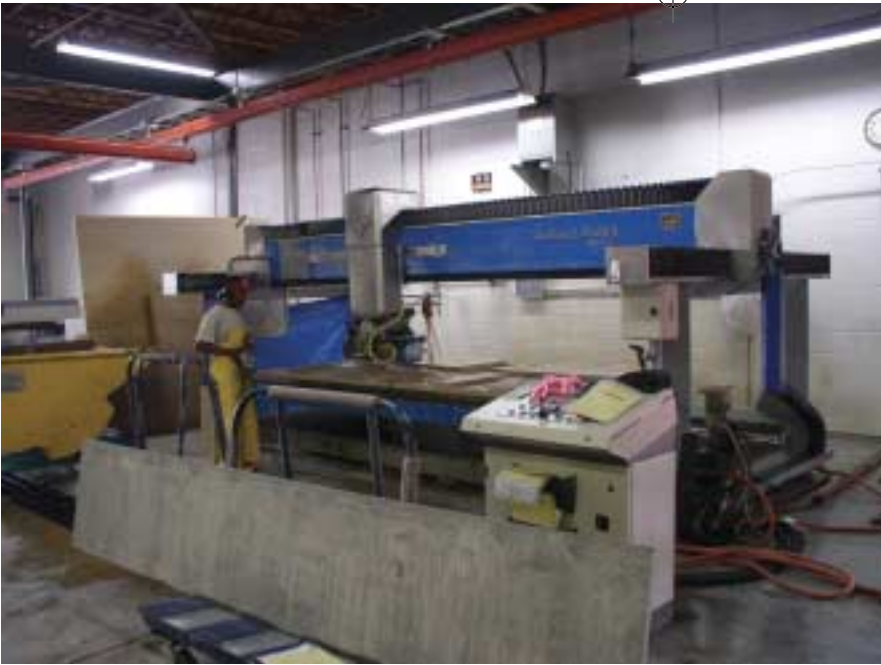
In the stone division, the fabricating shop is equipped with a Marmoelettromeccanica Dynamica bridge saw from Regent Stone Products.
