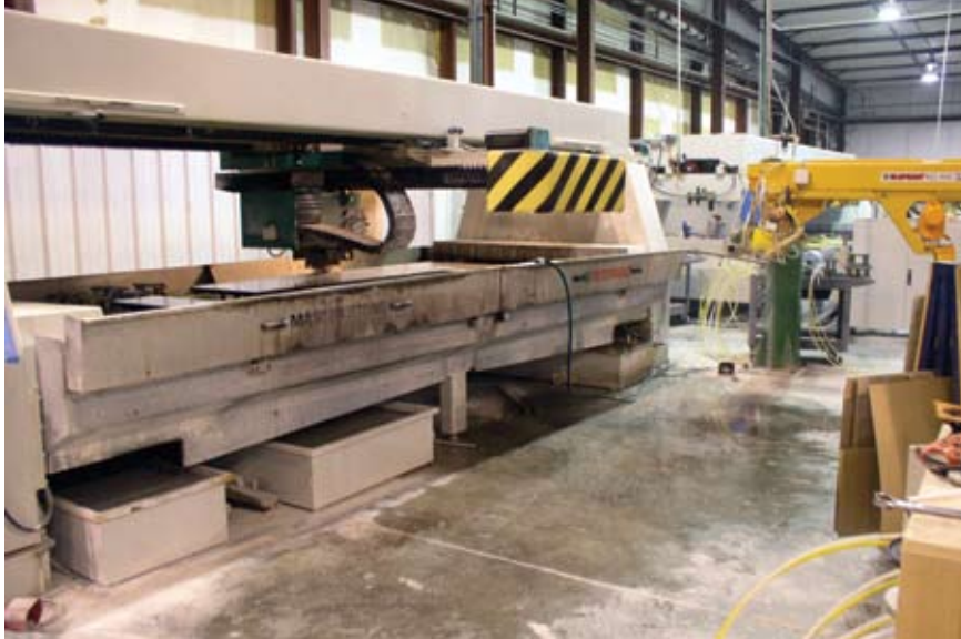
The stone shop is equipped with three Intermac Master Stone 4000 CNC machines from AGM.
