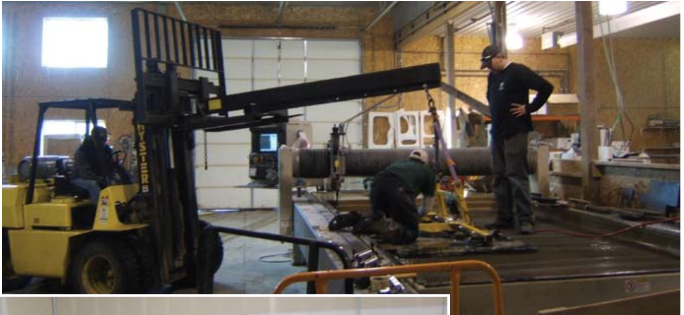
In total, Slabworks of Montana employs seven shop workers, who use vacuum lifters from Wood's Powr-Grip of Laurel, MT, to position slabs on the machines.
