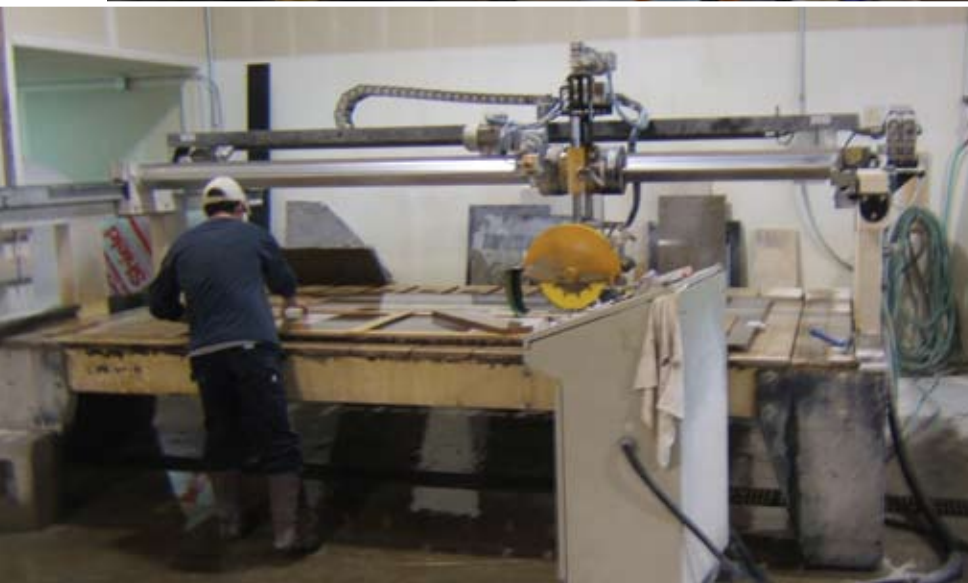
Two Achilli MBS-CE bridge saws, which were purchased from Braxton-Bragg of Knoxville, TN, are also used in the fabrication process.
